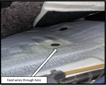
**Step 14:** Go under the vehicle and feed the door trigger signal wires (white and brown) and the disable switch wires (two black wires) into the cab. Feed the wires thru the hole in the rubber drain plug. Pop the drain plug back into the slot. Seal around the wires using RTV silicone adhesive to prevent water intrusion. These cables will run underneath the driver side seat.
