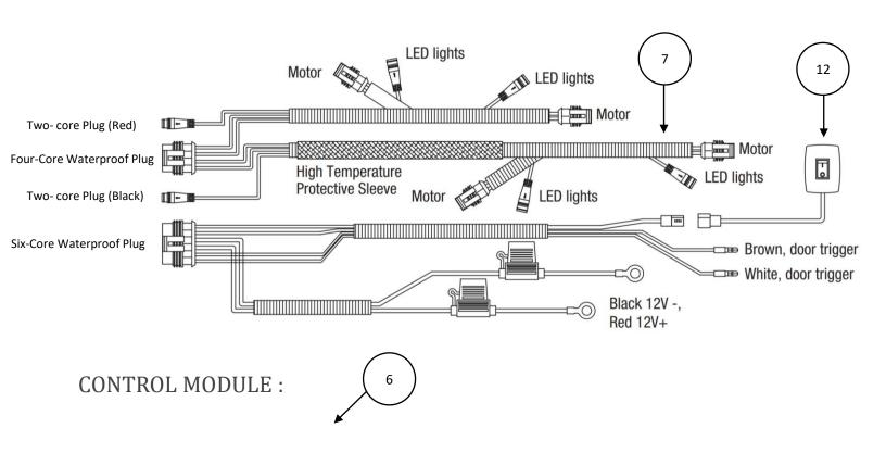
Notice: As shown in the picture, there is a four conductor plug, a six-conductor plug, a black two conductor plug, and a red two-conductor plug.
