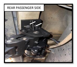
**Step 3**: Install the REAR DRIVER side motor using (2) M8X30mm Flange Bolts, to fasten the motor to the vehicle. The hardware should be hand tightened only until snug. This will allow the motor assembly to move and align easier when installing the running board.
