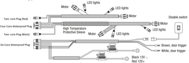
**Step 9:** Route the electrical harness from the controller along the frame rail of the vehicle. Connect the male plug connector on the wire harness into the female socket on the motors. The harness is labeled to show where to plug each male connector to the female connector. For example, Front Left is for the front Driver side motor and Rear Left for the rear Driver side motor. Use supplied zipties to secure harness to the frame rail.
