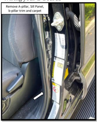
**Step 15:** Route the PASSENGER side door trigger wire (brown) towards the PASSENGER side b-pillar. Route the DRIVER side door trigger wire (white) and the black disable switch wires under the center console to the left side of the vehicle. The white wire needs to go to the driver side b-pillar, the black wires will go to the center console.
